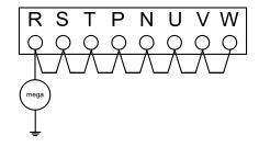
· Never test the withstand voltage on the inverter.
