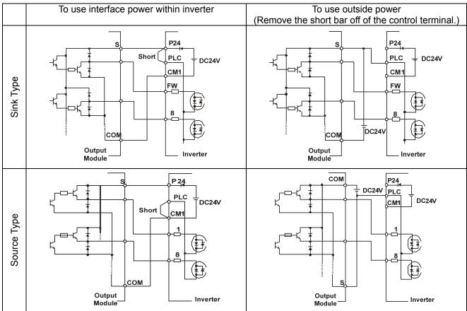
Fig 2-6 Input terminal and PLC connection
