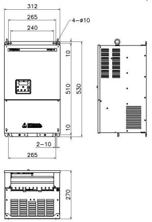
(4) N700E-450HF/550HFP, N700E-550HF/750HFP model external dimension.(mm)
