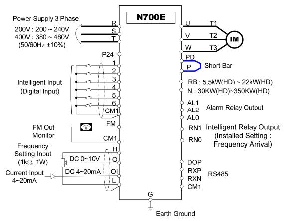
Fig 3-1 Setting diagram from the terminal control
