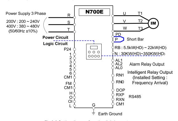
Fig 3-2 Setting diagram from the digital operator
