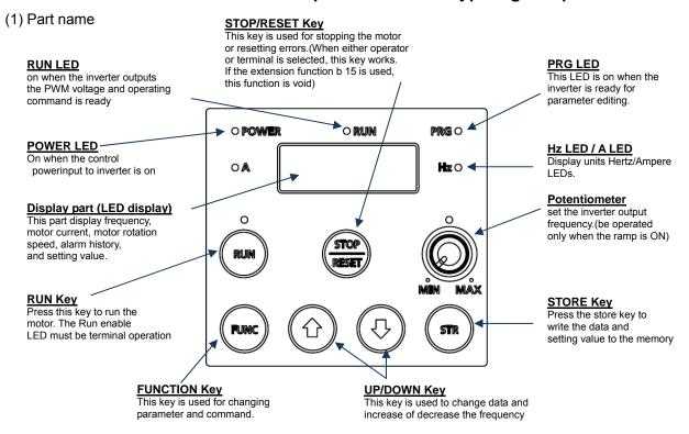
Fig.4-1 LED Type Digital Operator
