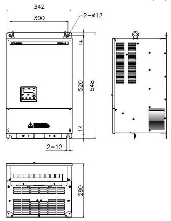
(5) N700E-750HF/900HFP, N700E-900HF/1100HFP model external dimension.(mm)
