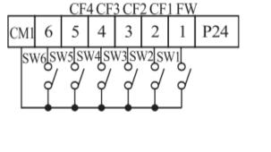
While using the multi-speed capability, you can monitor the current frequency with monitor function F01 during each segment of a multispeed operation.
