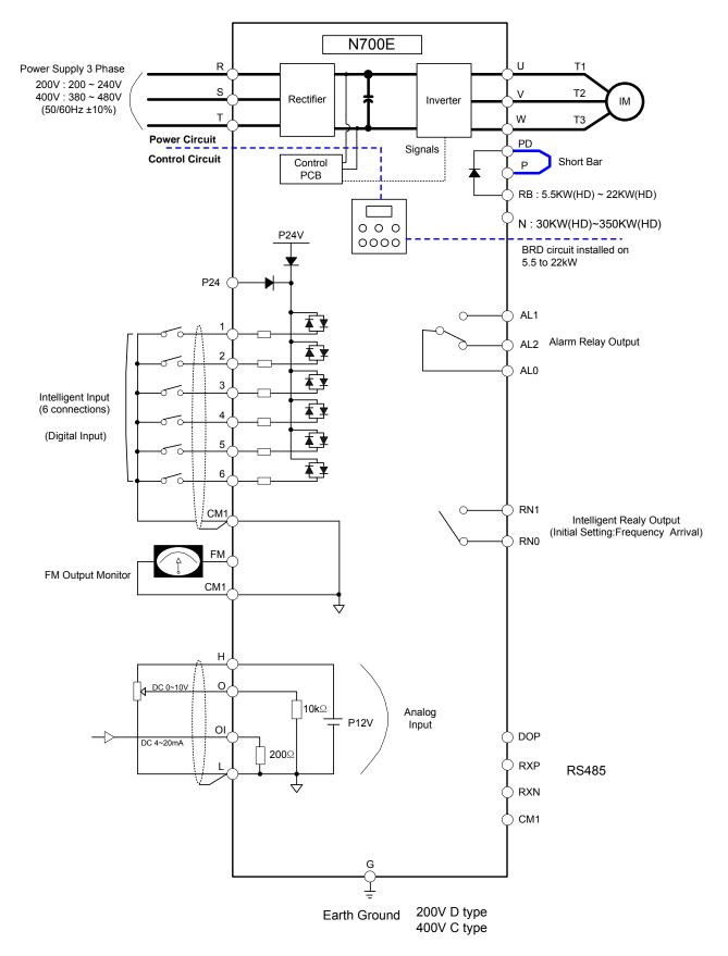
Fig.2-3 Terminal Connection Diagram (sink type)
