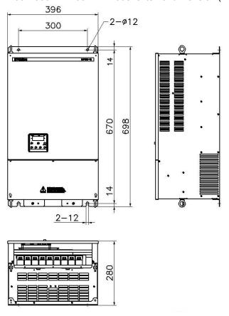
(6) N700E-1100HF/1320HFP, N700E-1320HF/1600HFP model external dimension.(mm)
