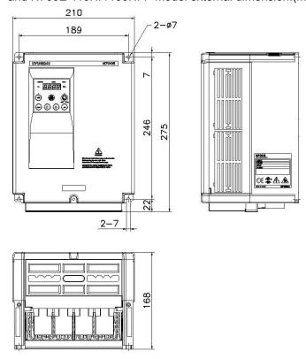
(2) N700E-150LF/185LFP, N700E-185LF/220LFP, N700E-220LF, N700E-150HF/185HFP, N700E-185HF/220HFP, N700E-220HF/300HFP model external dimension.(mm)
