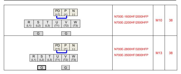
Table 2-3 Wiring of main circuit terminals
