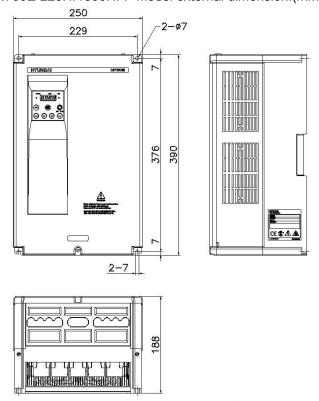
(3) N700E-300HF/370HFP, N700E-370HF/450HFP model external dimension.(mm)
