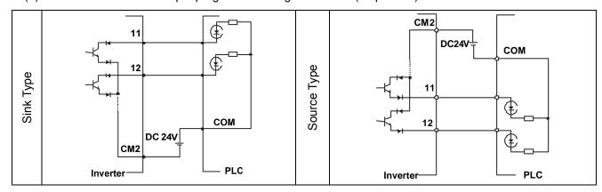
Fig 2-7 Output terminal and PLC connection
