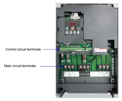
Fig1-4 Front cover removed
