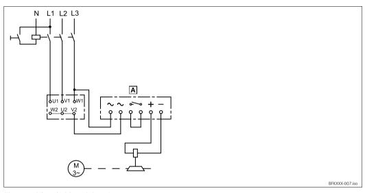
Fig. 14 AC switching, delayed engagement
