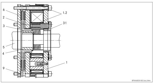
Design of the BFK468 spring-applied brake: basic module E (complete stator) + rotor + hub + Fig. 1 flange
