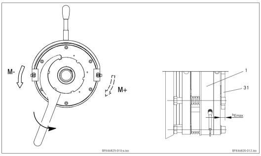
Fig. 18 Braking torque adjustment
