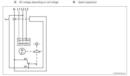
Fig. 17 With microswitch / wear check addition for all circuits; connection diagram also valid for star connection
