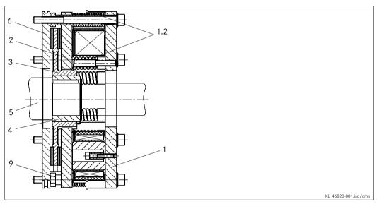
Fig. 2 Design of the BFK468 spring-applied brake: basic module N (complete stator) + rotor + hub + flange
