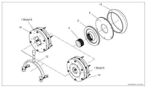
Fig. 19 BFK468-18 spring-applied brake to 31
