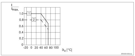
1 For screw assembly with metal surface (good heat dissipation)
